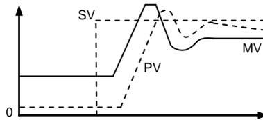
Figure 6-5 PID without Differential Forward
