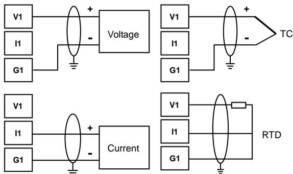
Figure 2-6 Analog input connection
