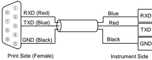
Figure 2-15 Connection between the instrument and the micro printer
