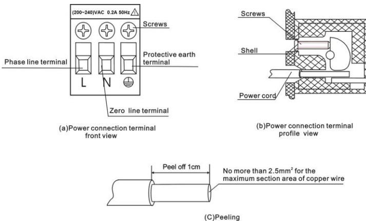
Figure 2-5 Power supply connection
