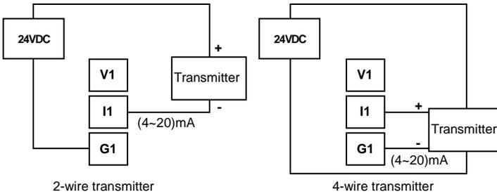
Figure 2-10 Transmitter power supply (External 24VDC) connection
