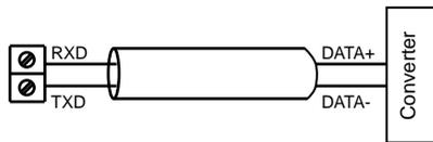
Figure 2-13 Connection between the instrument and the communication converter
