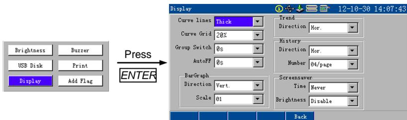
Figure 4-6 Display Setup
