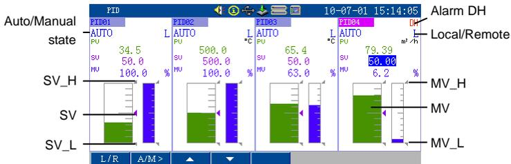
Figure 6-8 PID Display
