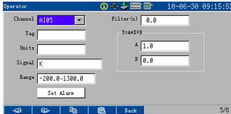
Figure 5-4 Channel Setting for TC Measurement
