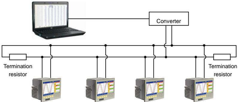
Figure 2-12 RS-485 communication between computer and several instruments
