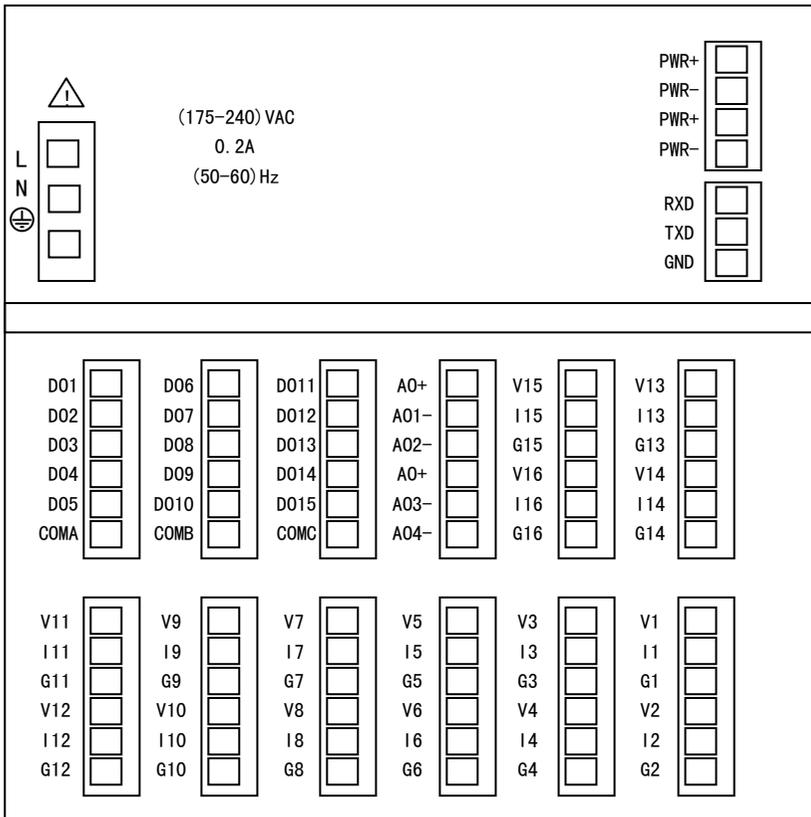
Figure 2-4 Terminal arrangement
