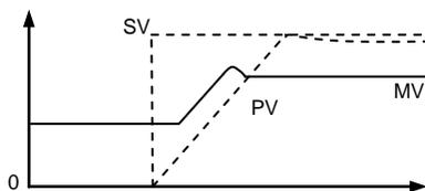
Figure 6-4 PID with Differential Forward
