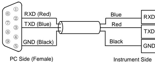
Figure 2-11 RS-232C communication between computer and the instrument
