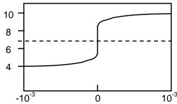
Figure 6-6 Process of pH neutralization
