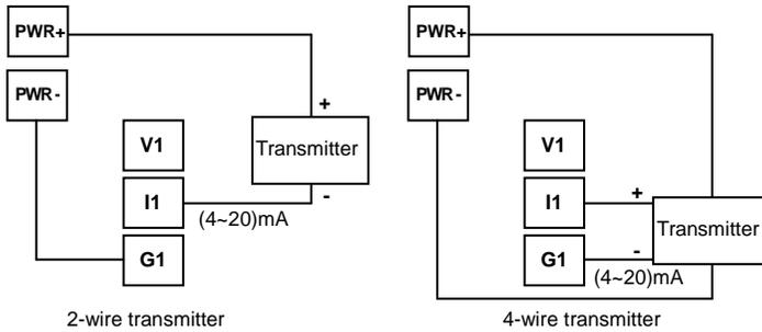
Figure 2-9 Transmitter power supply connection
