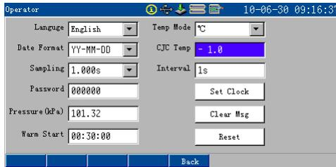
Figure 5-5 Cold Junction Compensation for TC Measurement
