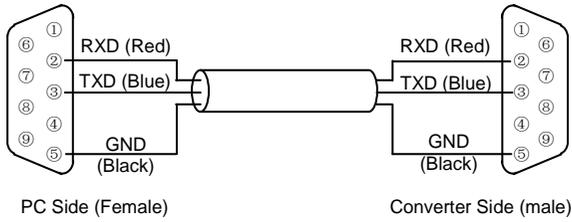
Figure 2-14 Connection between computer and the communication converter
